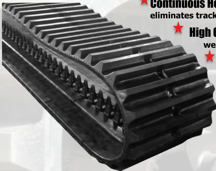
★ **Continuous Helically Wound Core Technology** - This technology eliminates track stretching and derailing.
